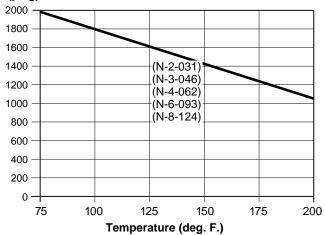
Suggested working pressures are 1/4 of burst pressure at system operating temperature.
