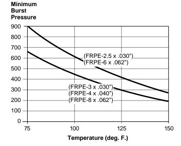
Suggested working pressures are 1/4 of burst pressure at system operating temperature.
